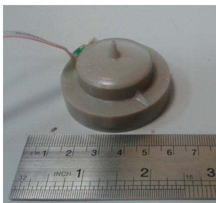
Figure 3. Appearance of a molecular electronic angular motion transducer.
