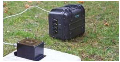
MTSS-1033A accelerometers (R-sensors) connected to TESTBOX-2010 digitizer (TDG)
