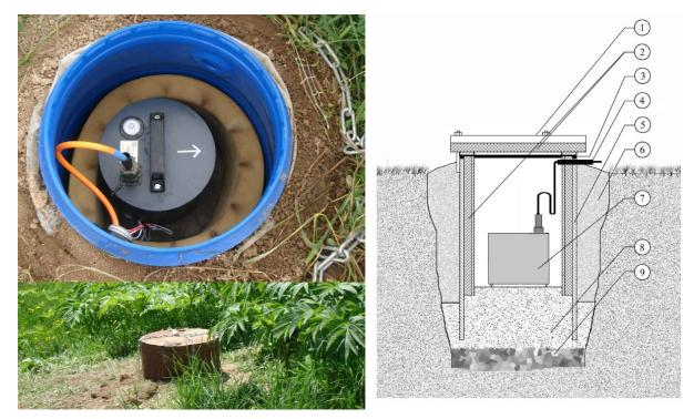
**Figure 2.** Equipment installation seismometer module (1. Module cover; 2. Heat insulation; 3. Sealing ring; 4. Input signal cable; 5. Module housing; 6. Filling; 7. CME-6111 seismometer; 8. Concrete base; 9. Crushed stone).
