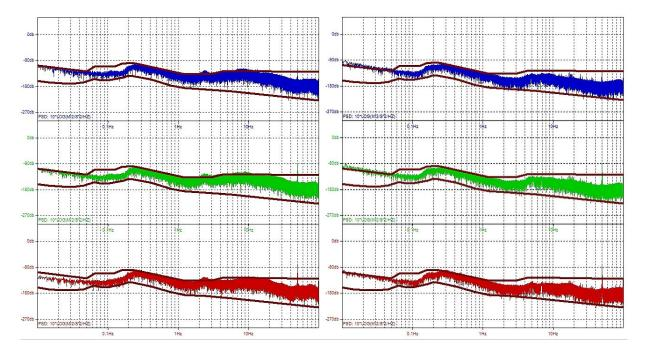
**Figure 4.** The spectral density of seismic noise of the CME-6111 seismometer (on the left - daytime, on the right – nighttime).
