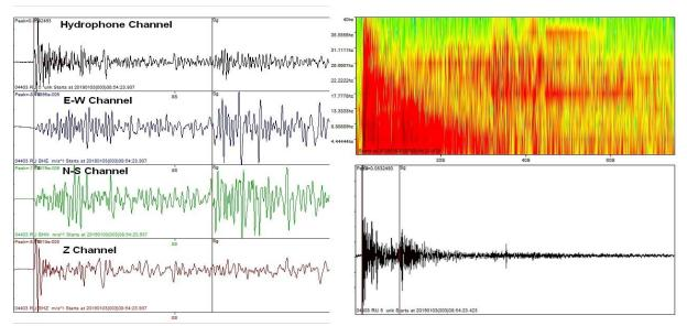
Figure 5. Recording a local seismic event with molecular electronic sensors. To the right is the spectrogram of this event, recorded by a hydrophone.
