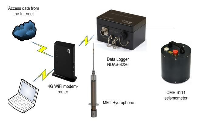
Figure 3. Equipment for seismic monitoring complex.
